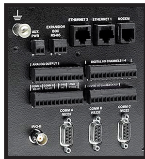
Switch Board Meter (Rear View)
